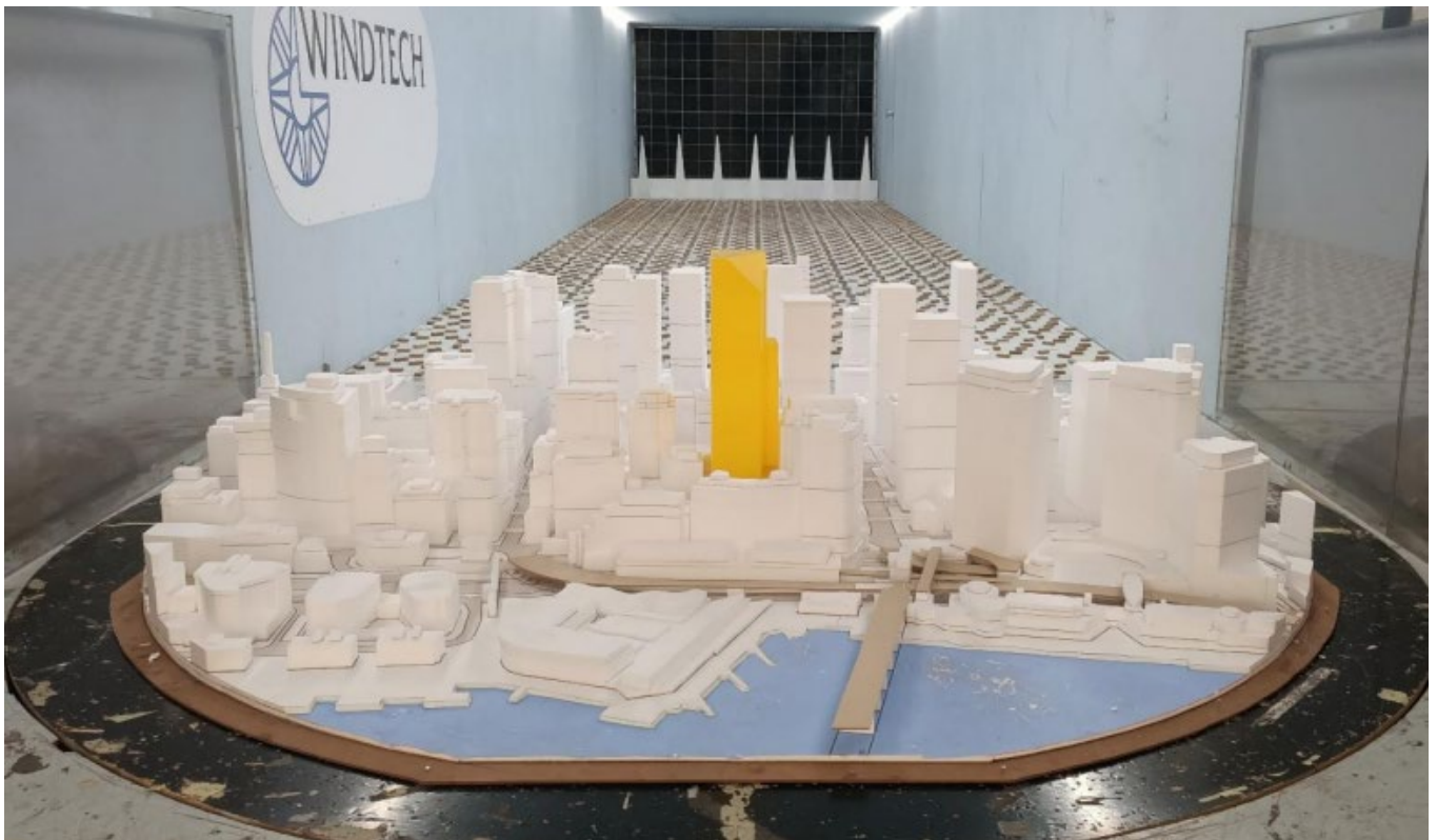
Figure 73 Wind Tunnel Modelling – Proposed Planning Envelope viewed from the west
